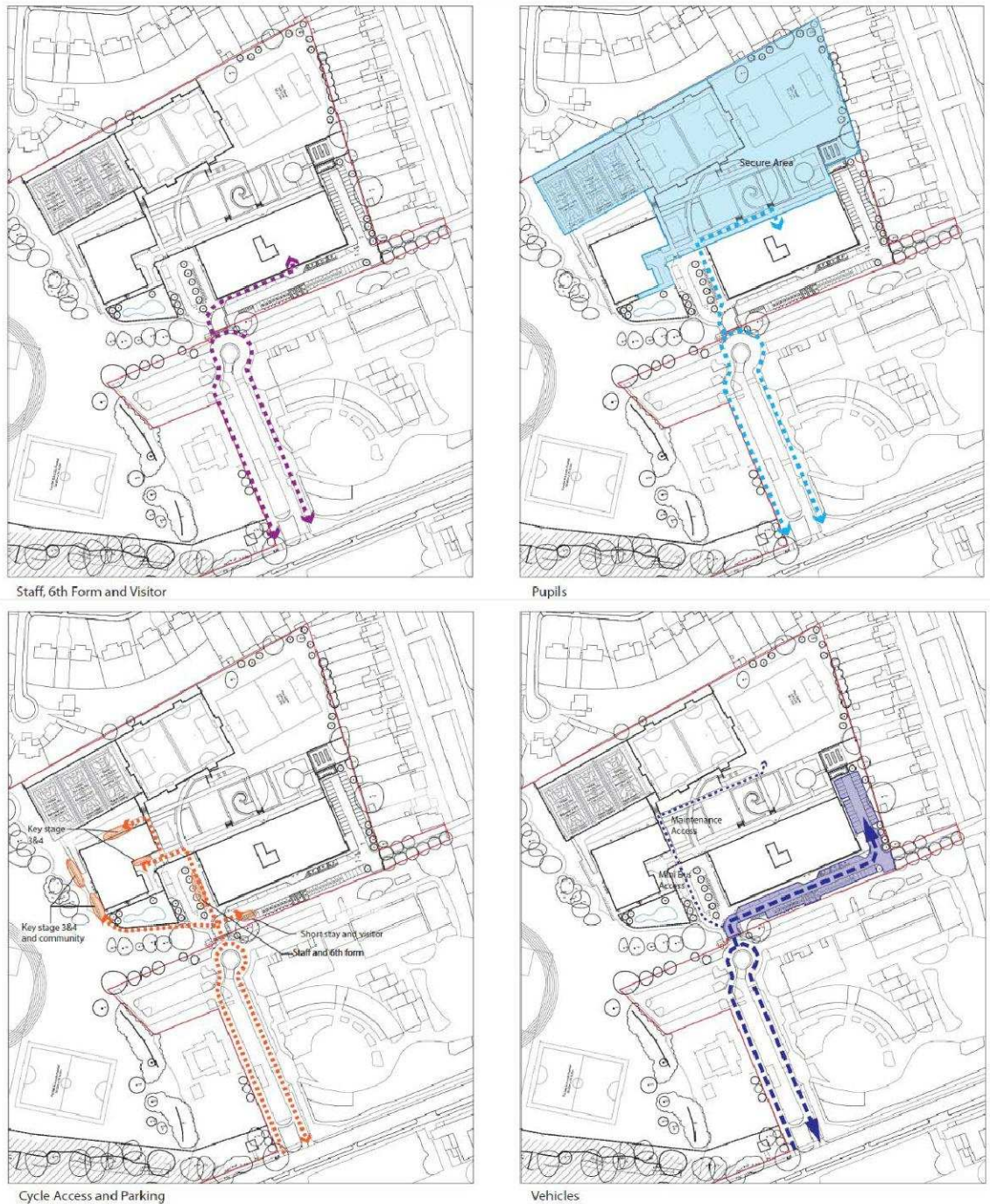
Figure 3 Site Layout, Movement & Access Arrangements
